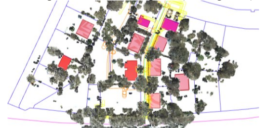
Figure 2: Compiled Model of The Pilot Area: Cadastral borders - blue; Milieu Zone - pink; Milieu Values – (red to light pink); Electricity network – Yellow, District Heating network – Orange; Road – Green; Trees
