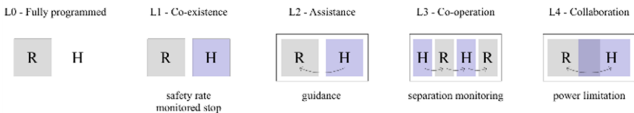
Figure 2: Levels of interaction in hybrid fabrication for construction. R = Robot and H = Human. Adapted from Mukherjee, et.al. (2022_
