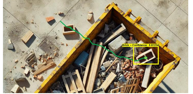
Figure 5: Example of tracking and detection of waste on a waste collection container.
