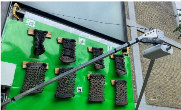
Figure 3: The EMA monitoring Rig follows the behaviour of BioPol panels over time.
