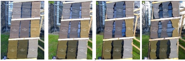
Figure 8: An image segmentation tools allow to track and quantify the deformation of each BioPol panel over time. In the screenshots from a stop motion animation the shrinkage of the nine biopolymer panels is visible from left to right.
