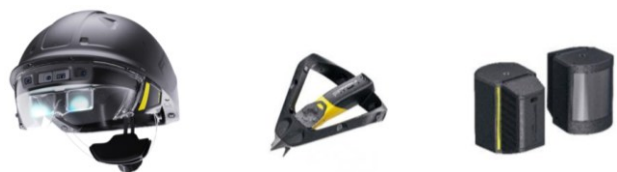
Figure 1: The AR headset (ATOM), the pointing device, and the tracking beacons.
