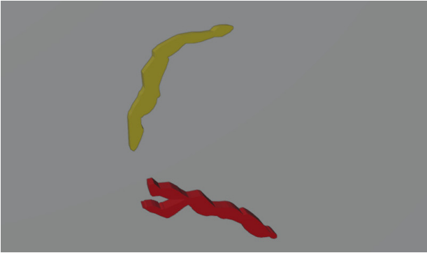
Figure 9: BIM object of detected crack.
