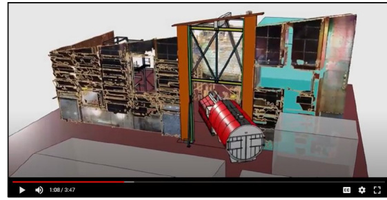
Figure 3: 4D simulation with BIM and point cloud to coordinate the transportation logistics of mechanical equipment at the BRDF project ©Kinetic Construction
